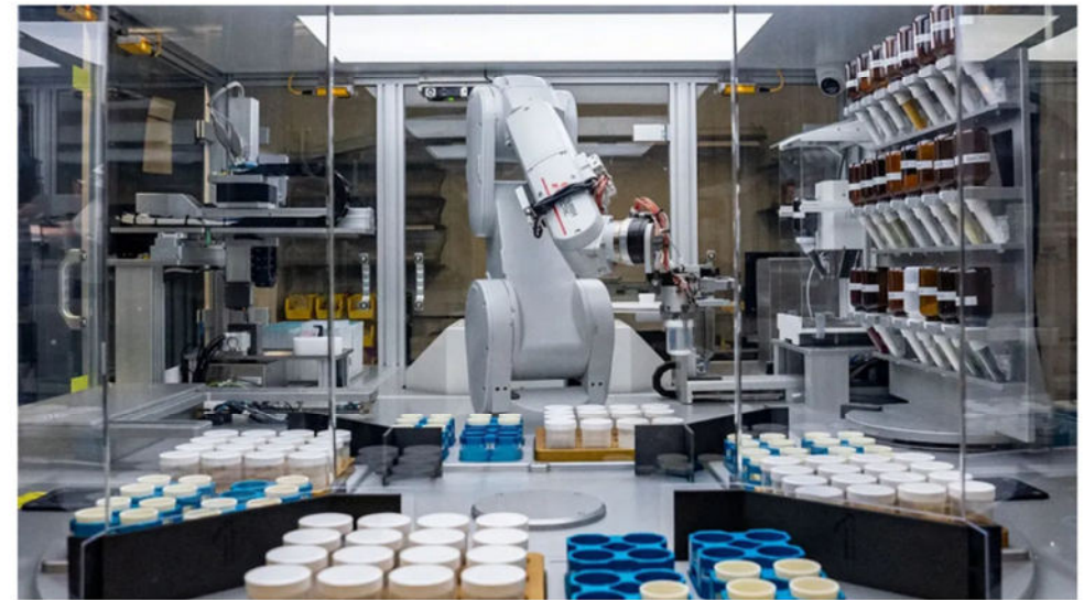
A-Lab, a facility at Berkeley Lab where artificial intelligence guides robots in making new materials. Photo credit: Marilyn Sargent/Berkeley Lab
